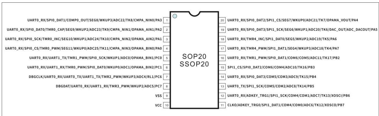
Figure 3-2 JSH3000 SOP20/SSOP20 package
